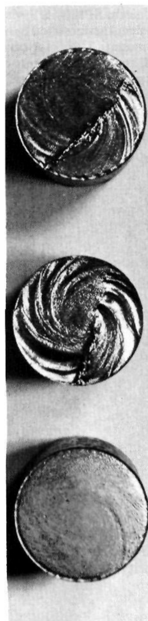
Figure 2. Relief structure on disk surfaces following reaction with cyclopentyl bromide in ether. (Top) Disk used in typical kinetic runs. Data obtained using this disk are included in Figure 5. The heavily etched line across the disk results from preferential etching close to a microscopic crack. The total quantity of alkyl bromide consumed by reaction of this disk (including 1,2-dibromoethane) was 12 mmol. (Center) A disk which had been allowed to react with 35–40 mmol of alkyl bromide. The etching in this disk was sufficient to produce an appreciable change in surface area. (Bottom) Uncracked disk, used to establish that the crack-associated etching obvious in the top disk had not distorted the observed rate constants. This disk was allowed to react with 12 mmol of alkyl bromide.
